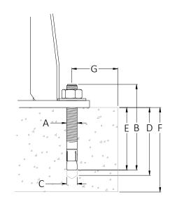
5/8 " 7 " • ANCHOR DIAMETER (A): ANCHOR LENGTH (B): ANCHOR DRILL (C): 5/8 " ANCHOR DRILL DÉPTH (D): 4 3/4" ANCHOR EMBEDMENT (E): 4 1/2 " 6" CONCRETE THICKNESS (F): MIN EDGE DISTANCE (G): 10" ANCHOR BOLT TORQUE: 80 ft-lbs
