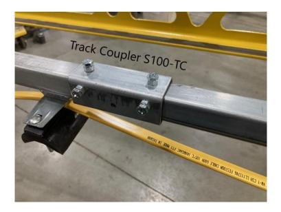
**1.3** Hold each festoon trolley and loosen the 2 bolts that hold the plastic clamp plate on the festoon trolley. Then roll the festoon trolleys into the festoon track without the festoon wire installed.
