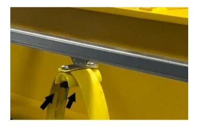
**1.4** On the end of the beam nearest where your power supply for this festoon will be, install the single bolt anchor hanger S100-AH with the anchor bolt on the side of it. Then install the festoon trolley clamp style S100-CET with bolts to the track as shown below.
