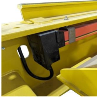
4.3.2 ElectroTrack Hanger Bolted Directly to Beam
