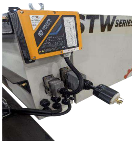
4.14.2 Radio Receiver Pre-Attached on Control Panel
