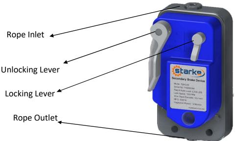
If it is necessary to lock the safety wire rope manually, turn the "Locking Lever" counterclockwise. A "click" indicates that the wire rope is locked by the wire rope locking mechanism.
